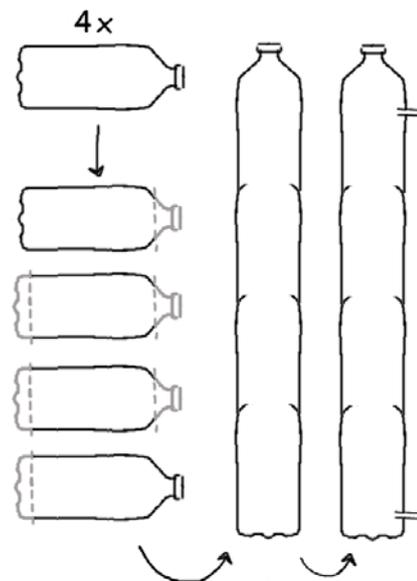
**Figure 2:** Sketch on how to cut the bottle and where to put the flexible tubes
