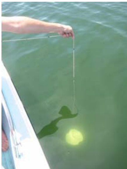
Fig. 2 Secchi disk measurement
